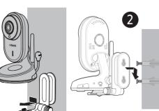
4. Place the baby unit on the wall mount bracket, and then slide it forward until it locks into place. Align the holes on the wall mount bracket with the screws on the wall, and slide the wall mount bracket down until it locks into place.
