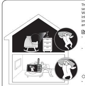
The baby unit has infrared LEDs that allow you to see your baby clearly at night or in a dark room. When the baby unit detects low light levels, the infrared LEDs are switched on automatically. The images from the baby unit are in black and white, and a appears on the parent unit screen.
