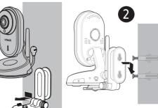
You can maximise your baby unit viewing angles by tilting the wall mount bracket. Hold the baby unit, and then rotate the knob in an anticlockwise direction. This will loosen the joint of the wall mount bracket. Tilt your baby unit up or down to adjust to your preferred angle. Then, rotate the knob in a clockwise direction to tighten the joint and
